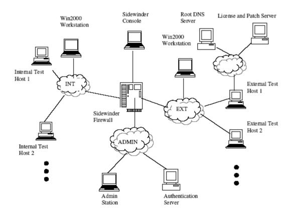
Developer test environment network diagram
