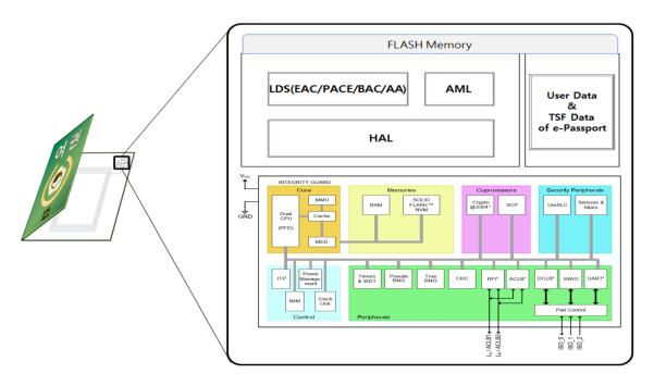
[Figure 1] Architecture of the TOE
