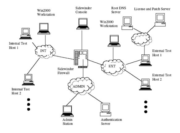
Developer test environment network diagram
