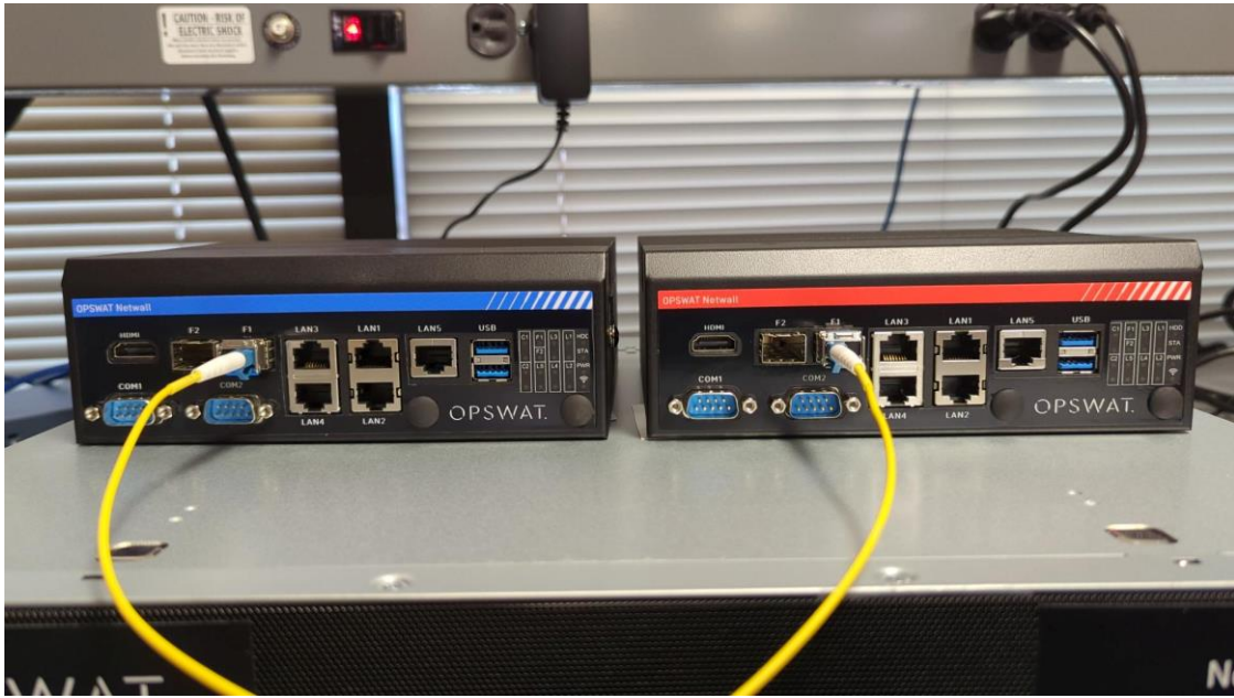
Figure 7 - OPSWAT NetWall Optical Diode Din Rail version
