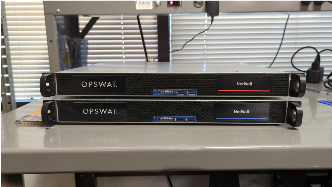
Figure 6 –OPSWAT NetWall Optical Diode 1U version
