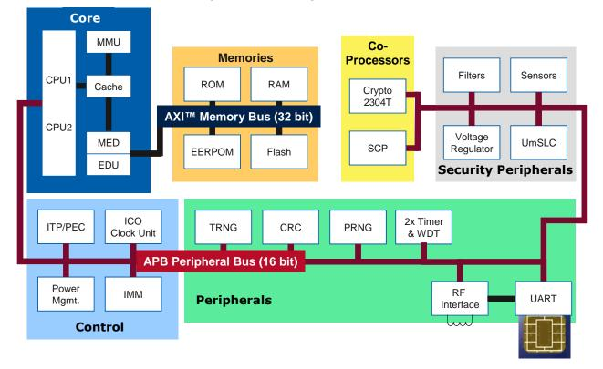
Figure 1: Block diagram of the TOE
