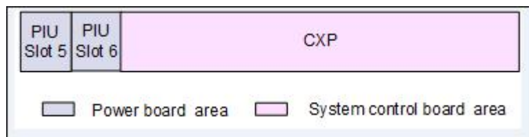
Figure 1-8 The functional host system of OptiX PTN 910E-F
