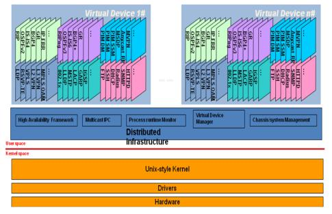
Figure 2: Comware V7.1 Module Design
