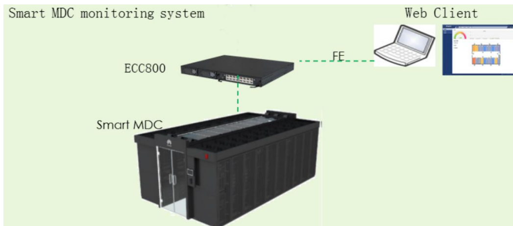
Figure 1-2 Position of the monitor controller on the smart modular data center
