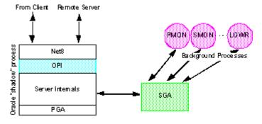
15. The Process Monitor provides process recovery when a process fails. The System Monitor provides database instance recovery and the Log Writer writes to the redo logs.
