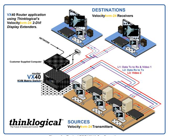
Figure 2a. Typical TOE VX40 Configuration
