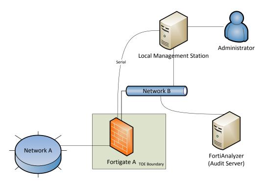
Figure 1 – TOE Physical Boundary
