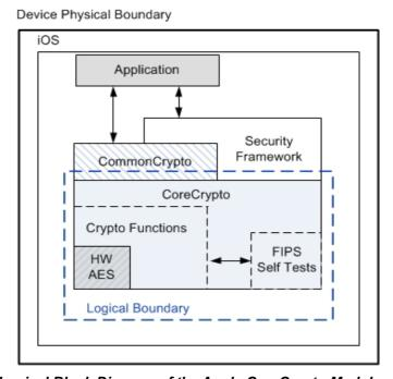
Figure 3: Logical Block Diagram of the Apple CoreCrypto Module v8 for ARM.
