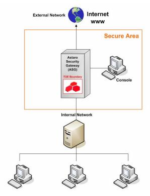
Figure 1: Typical ASG Network Configruation
