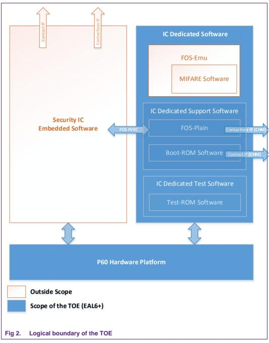
Fig 2 also shows that the FOS-Emu including the MIFARE Software is not part of the TOE.
