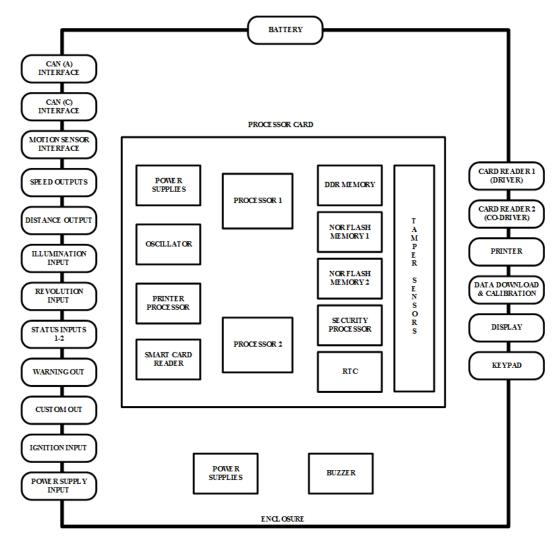
Figure 4: Aselsan Digital Tachograph Vehicle Unit
