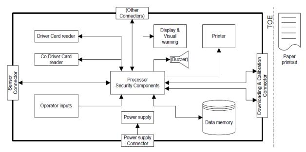
Figure 1: Block Diagram of the TOE
