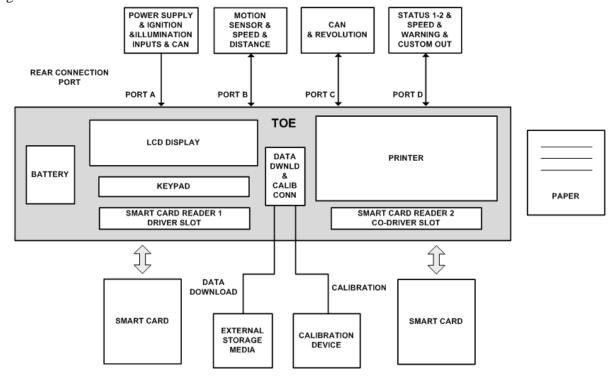
Figure 3: TOE Operational Environment
