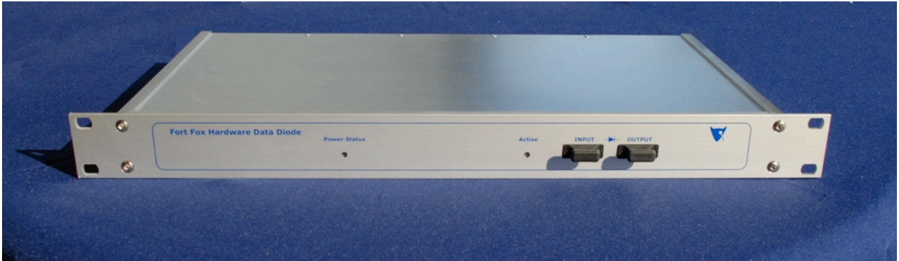
Figure 2: The TOE as a single 19" rack component
