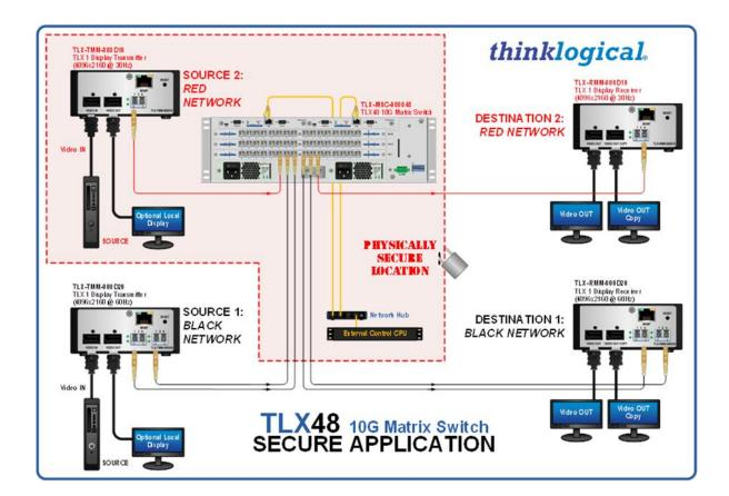
The figure shows the TLX48 Router KVM Matrix Switch in an evaluated configuration. An equivalent layout is the evaluated configuration for the TLX320 Router KVM Matrix Switch.
