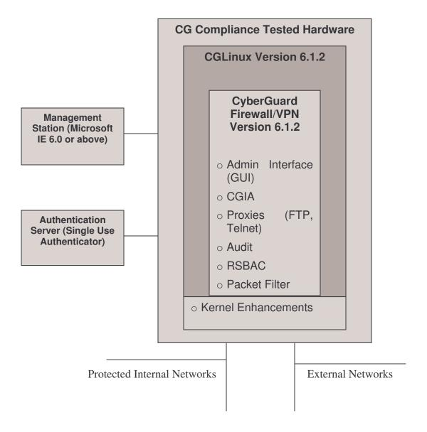
Figure 2 - TOE Physical Boundary
