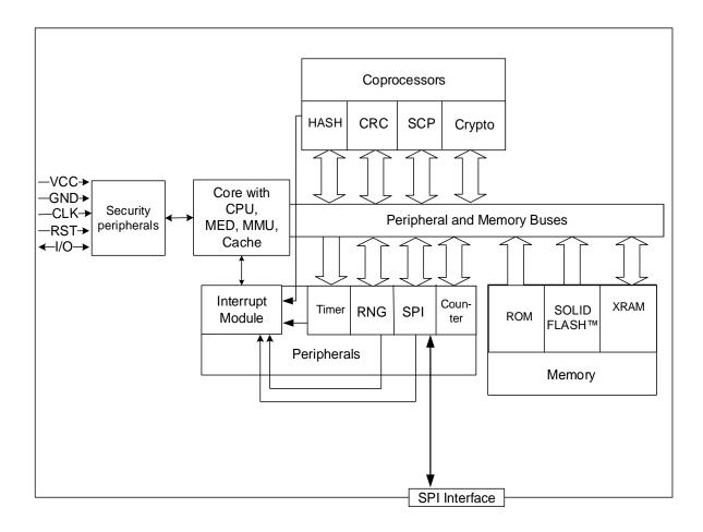
Figure 1: Block diagram of the SLB9670 2.0
