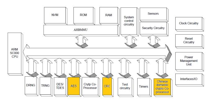
The hardware of the TOE has the following components:
