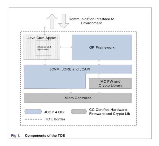
The TOE consists of an applet which is executed by a software stack that is stored on a Micro Controller. For a complete picture of the TOE see Fig 1, and for details with regards to the different components see section 1.3.5.
