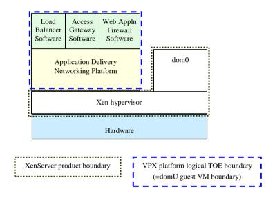
Figure 3: VPX Platform TOE detail
