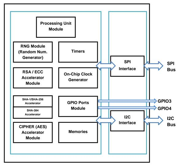
Figure 1 - TPM2.0 Block Diagram
