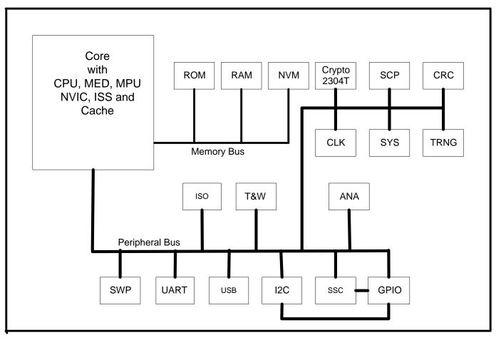
Figure 1: Block diagram of the TOE
