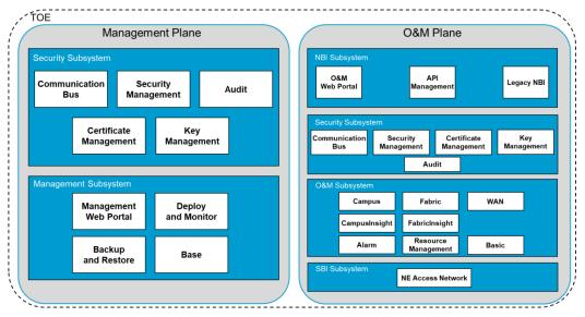
The TOE logical architecture consists of two independent planes, and each plane consists of a number of subsystems and modules:
