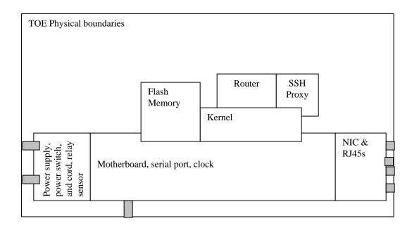
On power-up, the hardware boots the embedded operating system. At the end of its standard startup procedure, the the system starts the Router.
