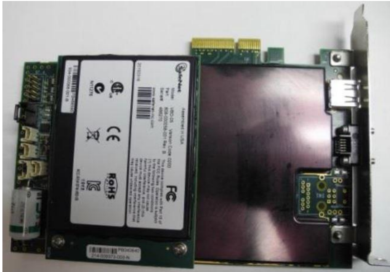
Figure 2 – Luna® PCI-E Cryptographic Module (TOE)
