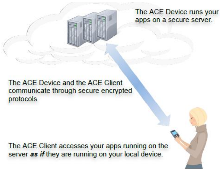
Figure 1 ACE Client as Part of VMI Platform
