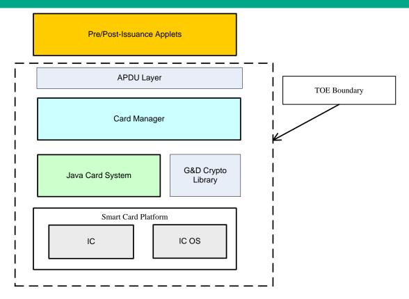
Figure 1: TOE boundary (dotted line)
