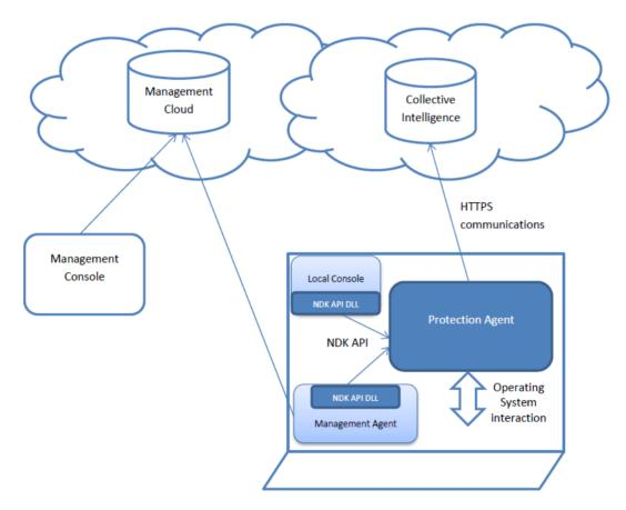
The TOE, marked as dark blue, is composed of the Protection Agent, which implements the main TOE security functionality (process interception, risk analysis, audit functionality, etc), and the NDKAPI DLLs, which provide an ease-of-use API, using an encrypted channel, to other Panda processes in order to receive notifications and user logs from the Protection Agent and to manage the Protection Agent itself.
