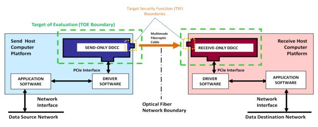
Figure 4: TOE Architecture
