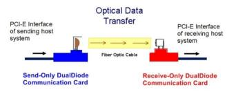
Figure 3 – High Level view of the DualDiode Interface
