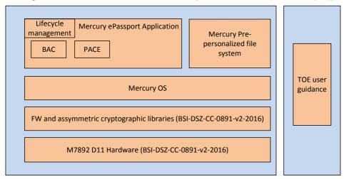
Figure 1. Logical architecture of the TOE.
