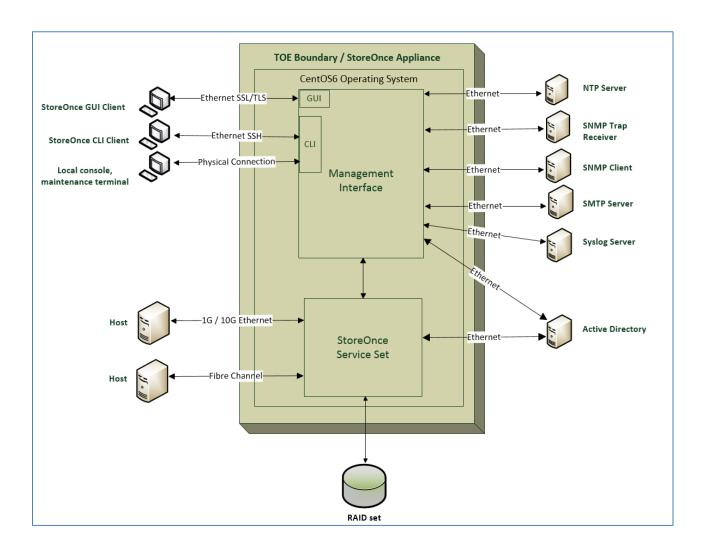
Figure 1 TOE Architecture
