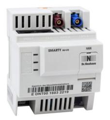
Figure 3: SMARTY IQ-SMGW casing and external interfaces
