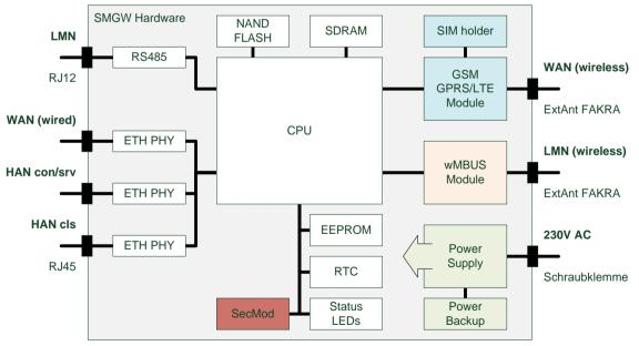
Figure 4: SMARTY IQ-SMGW internal structure
