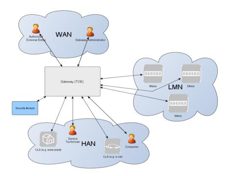
Figure 1: The TOE and its direct environment
