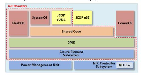
According to the *[ETR]*, the TOE is the eUICC Application on top of the Java Card Operating System and the SN300 Secure Element (including Dedicated Software) on which it is running. TOE identification provided in the ST identifies the JCOP 7.x OS with eUICC functionalities and including
