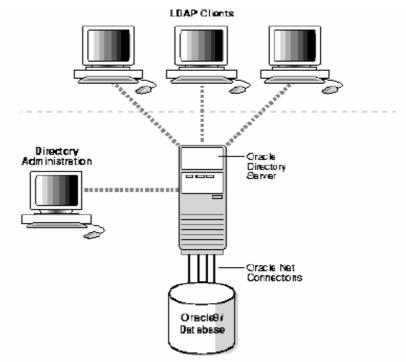
7. OID communicates with the database using ONS, which is Oracle's operating systemindependent database connectivity solution.
