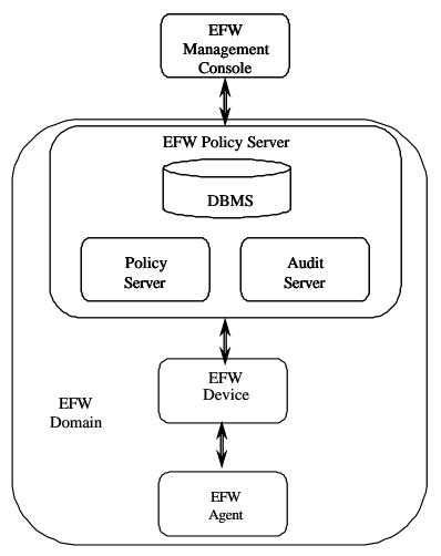
Figure 2 EFW Architectural Components
