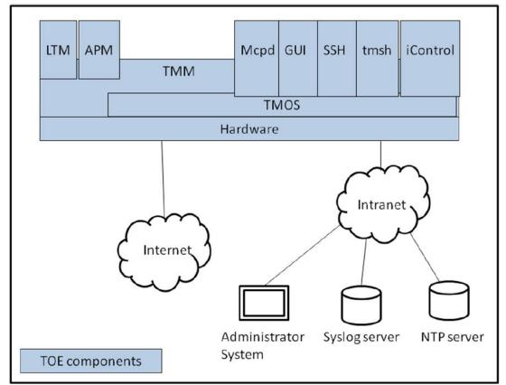
The TOE is separated into two distinct planes, the control plane and the data plane. The control plane validates, stores, and passes configuration data to all necessary systems. It also provides all administrative access to the TOE. The data plane passes user traffic through the TOE.
